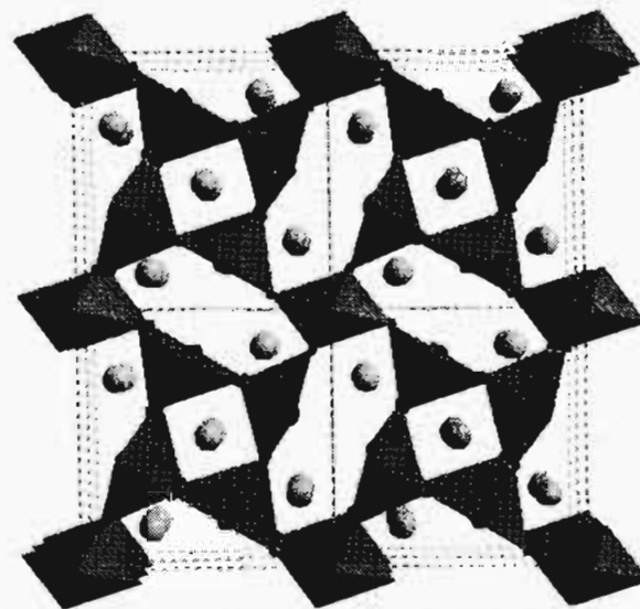
Figure 6. Structure of \text{NdCuO}_{2.6} projected on [001]. Large, medium, and small balls represent Nd, Cu, and O atoms, respectively.
