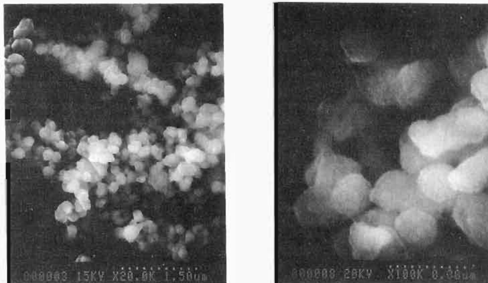
Figure 4. Scanning electron micrograph of ZnS produced by reaction of ZnS_6(TMEDA) with PBu_3 . The magnification is 20000 \times and 100000 \times , respectively.
