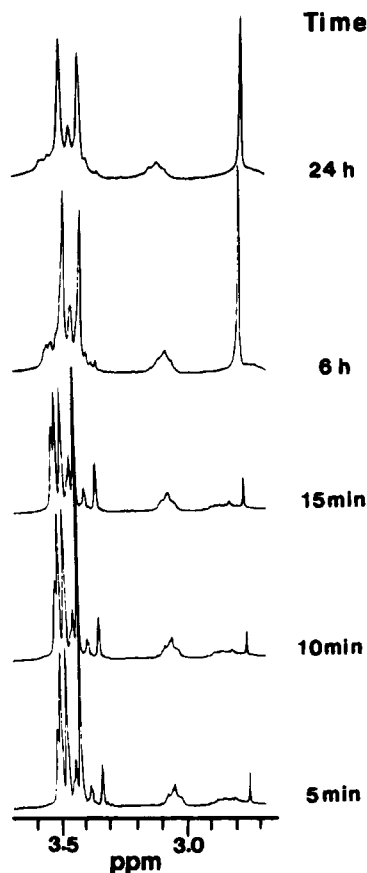
Figure 3. Hydrolysis with time of cis, fac -[RuCl 2 (Me 2 SO) 3 (NH 2 (CH 2 ) 4 -NH 3 Cl)], II , monitored by 1 H NMR spectroscopy.
