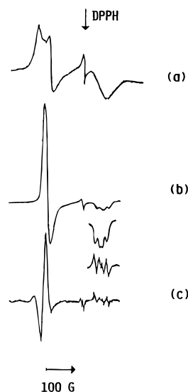
Figure 8. X-band EPR spectra of 5 under the following experimental conditions: (a) microcrystalline powder at T = 100 K; (b,c) \text{CH}_2\text{Cl}_2 solution at T = 100 K, first-derivative mode and second-derivative mode, respectively.
