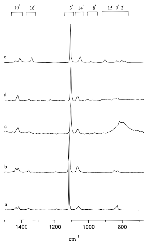
Figure 3. Raman spectra in the 700–1500 \text{cm}^{-1} region of (a) \text{Cp}_2\text{Fe}_2(\text{CO})_4 trans isomer, (b) \text{Cp}_2\text{Fe}_2(\text{CO})_4 cis isomer, (c) \text{Cp}_2\text{Mo}_2(\text{CO})_6 , and (d) \text{Cp}_2\text{W}_2(\text{CO})_6 , (e) \text{Cp}_2\text{Ni}_2(\text{CO})_2 . The broad absorption in c at ca. 800 \text{cm}^{-1} is due to fluorescence.
