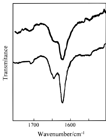
Figure 4. HOH bending region in the spectrum of isotopically isolated H 2 O molecules in practically perdeuterated Cs 2 [CrCl 2 (H 2 O) 4 ]Cl 3 : (Top) room temperature; (bottom) liquid-nitrogen temperature.
