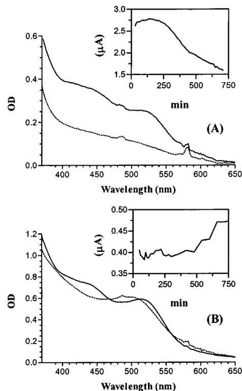
**Figure 1.** (A) UV–visible spectrum of **1** adsorbed onto optically transparent TiO<sub>2</sub> before (—) and after (···) overnight photolysis while immersed in propylene carbonate 0.1 M in NaClO<sub>4</sub>. (B) As in A before (—) and after (···) photolysis while immersed in 2-propanol. The insets show the measured photocurrents during the same periods.
