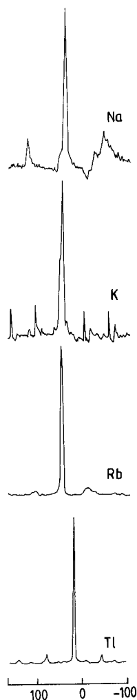
Figure 4. ^{27}\text{Al} MAS NMR spectra of \text{A}_3\text{Al}_2\text{P}_3\text{O}_{12} (A = Na, K ( 1 ), Rb ( 2 ), Tl ( 3 )) compounds.
