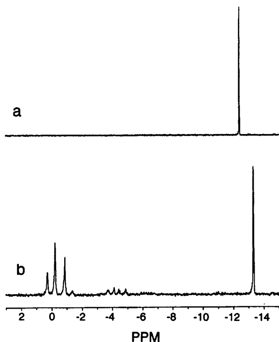
Figure 10. ^{31}\text{P} NMR spectrum of (a) H1 (0.01 M) in MeCN and (b) \text{H}_3\text{PW}_{11}\text{TiO}_{40} in \text{H}_2\text{O} (pH 1.8), both 24 h after the addition of a 100-fold molar excess of \text{H}_2\text{O}_2 .
