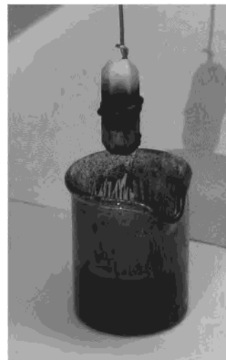
Figure 8. Photograph of a Teflon-coated stir bar magnet separating the room-temperature V[TCNE]_x \cdot yCH_2Cl_2 magnet after preparation.
