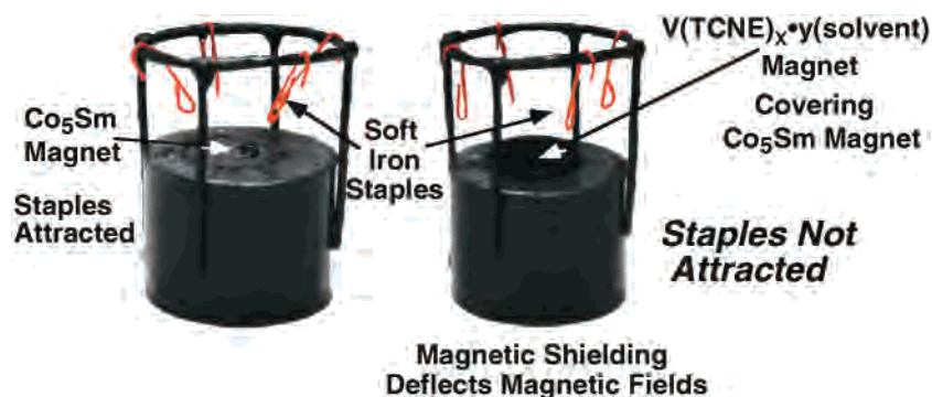
Figure 13. Illustration of the V(\text{TCNE})_x \cdot y(\text{CH}_2\text{Cl}_2) magnet being an effective magnetic shield at room temperature. Rods (paper clips) of soft-iron (red) are attracted to a \text{Co}_5\text{Sm} permanent magnet (left) when a 1.7 mm pellet of V(\text{TCNE})_x \cdot y(\text{CH}_2\text{Cl}_2) placed between the \text{Co}_5\text{Sm} magnet and the rods (red) hang freely (right), demonstrating magnetic shielding. 40
