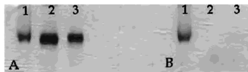
Figure 4. Native polyacrylamide gel electrophoresis stained (A) for protein using Coomassie Blue and (B) for cobalt using 1-nitroso-2-naphthol. Lane 1 is ferritin containing a core of Co(O)OH, lane 2 is apo-ferritin, and lane 3 is native ferritin containing an Fe(O)OH core.
