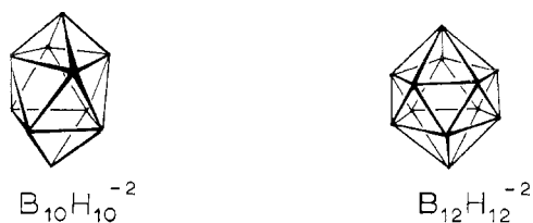
Figure 1.—The boron cage structure in B_{10}H_{10}^{-2} and B_{12}H_{12}^{-2} ions. Boron atoms are located at the corners.
