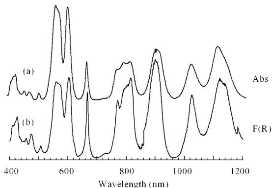
**Figure 2.** UV/vis/near-IR spectra for  $[\text{Pu}(\text{H}_2\text{O})_9][\text{CF}_3\text{SO}_3]_3$ : (a) in 1 M triflic acid solution; (b) diffuse reflectance of neat ground single crystals.
