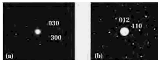
Figure 3. SAED patterns showing (a) [001] and (b) [221] projections of Sr 3 NaSbO 6 .
