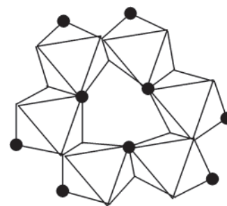
Figure 2. Schematic representation of the six VO 6 octahedra. Black circles denote the oxygen atoms that are hydrogen bonded to the \mu_6 -sulfato group. hydroxo), are somewhat longer than those reviewed by Khan and Zubietta. 5
