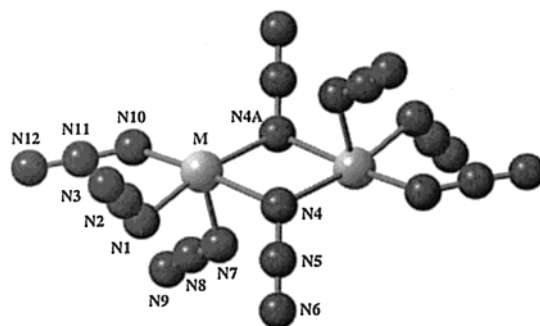
Figure 4. B3LYP-optimized structure of dimeric M(N 3 ) 4 - anions (M = As, Sb).
