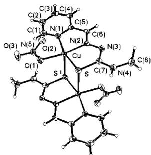
**Figure 1.** ORTEP plot of **1**. Selected bond distances (Å) and angles (deg): Cu–N2 1.964(2), Cu–O1 1.990(2), Cu–N1 2.028(2), Cu–S 2.2699(6), Cu–S' 2.7659(6), S–C7 1.759(2), N2–C6 1.291(3), N2–N3 1.358(2), N3–C7 1.333(3), N4–C7 1.325(3), N4–C8 1.454(4), N1–Cu–S 164.77(6), N2–Cu–O1 169.78(7), N1–Cu–S' 92.44(5), intramolecular Cu···Cu<sup>1</sup> distance 3.4482(2), closest intermolecular Cu···Cu distance 5.7498(4); Cu–S–Cu<sup>1</sup> 85.83(2) ( $I = -x + 1, -y, -z$ ).
