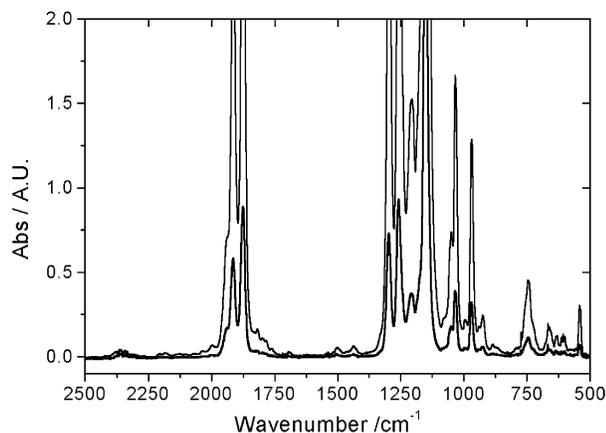
**Figure 1.** IR spectra of  $\text{CF}_3\text{OC}(\text{O})\text{OOC}(\text{O})\text{F}$  in the gas phase. Pressures are 2 and 8 mbar.
