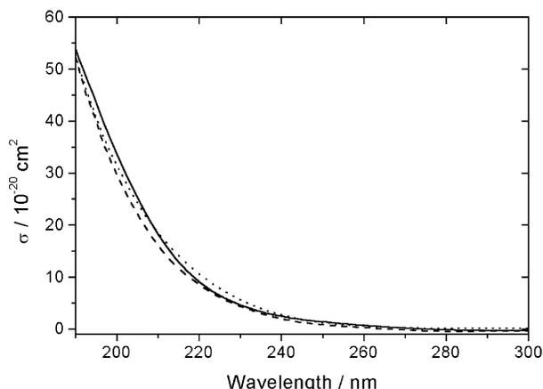
**Figure 3.** Absorption cross sections for gaseous  $\text{CF}_3\text{OC(O)OOC(O)F}$  (solid line),  $\text{FC(O)OOC(O)F}$  (dashed line), and  $\text{CF}_3\text{OC(O)OOC(O)OCF}_3$  (dotted line).
