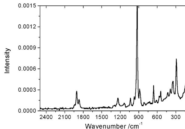
**Figure 2.** Room-temperature Raman spectrum of liquid  $\text{CF}_3\text{OC}(\text{O})\text{OOC}(\text{O})\text{F}$ .**Table 2.** Observed and Calculated Vibrational Wavenumbers
