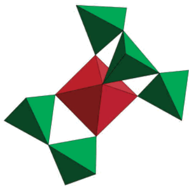
Figure 1. Structural motif ZrGe 5 present in the four structures ASU- n ( n = 23, 24, 25, 26), Ge tetrahedra green, Zr octahedron red.
