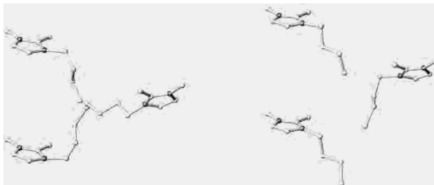
Figure 7. Section of the structure of butyldimethylimidazolium chloroferrate(II,III) showing the disordered butyl chains at 213 K (left) and 298 K (right). Each of the three crystallographically equivalent cations is shown with a different conformation of the butyl chain. The site occupation factors for the three conformations have been refined.
