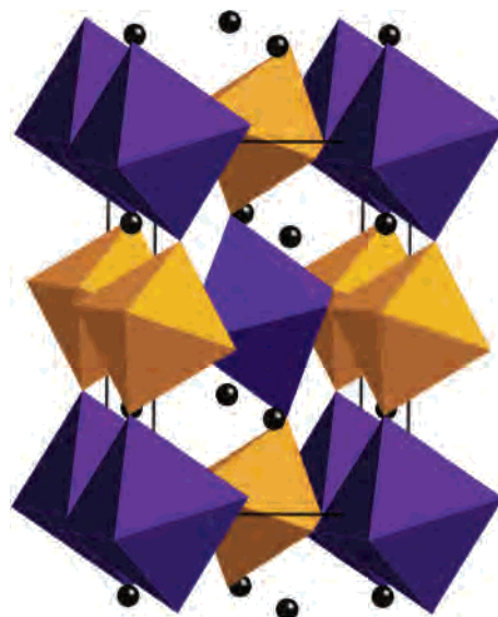
Figure 1. Crystal structure of \text{Ln}_2\text{NaOsO}_6 ( \text{Ln} = \text{La}, \text{Pr}, \text{Nd} ); \text{OsO}_6 octahedra are shown in orange, \text{NaO}_6 octahedra are purple, and the black spheres represent \text{Ln}^{3+} cations.
