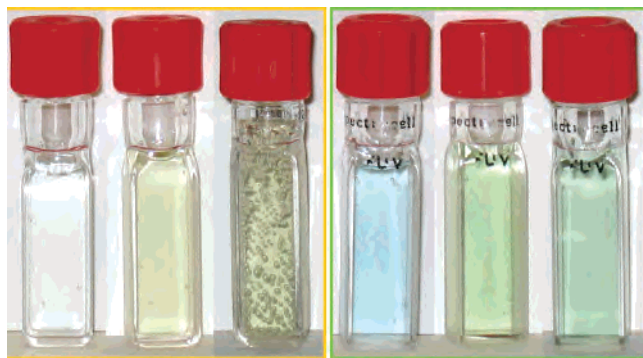
Figure 2. Visual changes in acidic solution, from left to right: 12 mmol L -1 Eu 2+ ; 12 mmol L -1 Eu 2+ with 0.3 mmol L -1 MeReO 3 after 1 min; 30 min later, showing hydrogen evolution; 12 mmol L -1 Cr 2+ ; 12 mmol L -1 Cr 2+ with 0.3 mmol L -1 MeReO 3 after 1 min; 1 h later. All solutions contain 120 mmol L -1 HCl.
