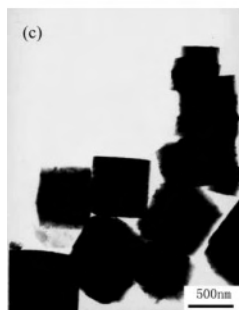
Figure 4. FESEM (a, b) and TEM (c) images of cubic FeS 2 crystallites obtained at 180 °C.
