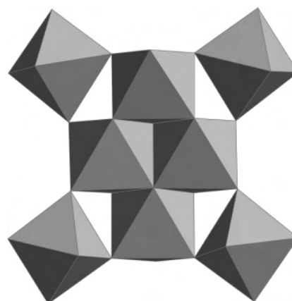
Figure 2. Polyhedral representation of the eight \text{AlO}_6 octahedra, of which the central four octahedra are edge-shared and the four peripheral octahedra are corner-shared.
