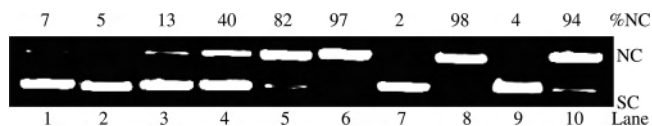
Figure 4. Cleavage of supercoiled pUC19 DNA (33 \mu\text{M} ) by [\text{Cu}(\text{py}_2\text{-phe})\text{B}](\text{ClO}_4)_2 (B = phen, 1 ; dpq, 2 ; dppz, 3 ; 40 \mu\text{M} ) using 3-mercaptopropionic acid (MPA, 5 mM) as a reducing agent in the presence or absence of additives in a 50 mM Tris-HCl/NaCl buffer (pH 7.2) at 37 ^\circ\text{C} containing DMF (10%): lane 1, DNA control; lane 2, DNA + 3 ; lane 3, DNA + MPA; lanes 4–6, DNA + complexes 1–3 , respectively, + MPA; lane 7, DNA + distamycin (100 \mu\text{M} ) + 2 + MPA; lane 8, DNA + distamycin (100 \mu\text{M} ) + 3 + MPA; lane 9, DNA + DMSO (2 \mu\text{L} ) + 3 + MPA; lane 10, DNA + \text{NaN}_3 (100 \mu\text{M} ) + 3 + MPA.
