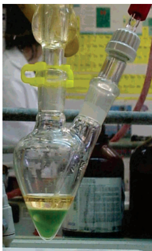
Figure 3. The initial biphasic system at RT with the upper chlorobenzene layer and the perfluoroheptane lower layer containing precatalyst 1 .
