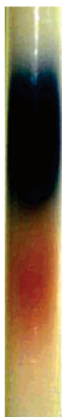
Figure 3. Photograph of the Sephadex G-50 column taken just a few minutes after the sample mixture was charged. Two distinct colored bands have already separated and correspond to \text{Mo}_2\text{VP}_2\text{W}_{15} (blue) and 1 (pink), with the latter eluting first.
