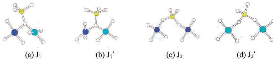
Figure 5. Intrachain spin dimers of Rb 2 Cu 2 (MoO 4 ) 3 associated with the spin-exchange paths (a) J_1 , (b) J_1' , (c) J_2 , and (d) J_2' .
