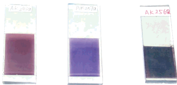
Figure 3. Thin film of anatase TiO 2 coated on FTO glass impregnated with dye 13b (left), 14b (middle), and 15b (right).
