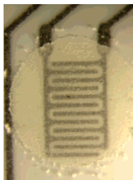
Figure 7. Homogeneous sensor layer formed from material A ( \text{Bi}_2\text{MoO}_6 (70%)/ \text{Bi}_2\text{Mo}_2\text{O}_9 (30%)).
