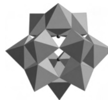
Figure 1. Polyhedral representation of 1 , the \alpha -Keggin structure, consisting of four sets of three edge-shared \text{WO}_6 octahedra or triads linked together by shared corners. This \text{W}\text{--}\text{O} framework encloses a central cryptand cavity defined by four internal \mu_3 -bridging O atoms, one from each triad, arranged in a tetrahedron about the anion center with overall T_d symmetry for the formal \alpha\text{-}[\text{W}_{12}\text{O}_{40}]^{8-} unit. The two protons (blue) are coordinated to and rapidly exchange among the four equivalent internal O atoms, thus preserving the T_d symmetry of the anion on the NMR time scale, as is consistent with the ^1\text{H} , ^{17}\text{O} , and ^{183}\text{W} NMR spectra of 1 in an aqueous solution. 6,10
