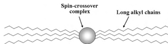
Figure 1. Construction of the metallomesogen with spin-crossover phenomenon.
