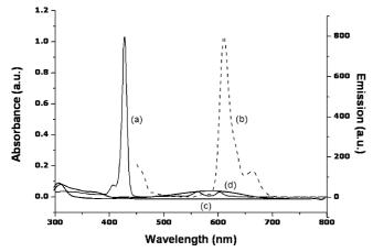
**Figure 1.** (a) UV–vis absorption and (b) fluorescence spectra of **Sn**(**T**-**TP**)(**OH**)<sub>2</sub>, UV–vis absorption spectra of (c) free **DTE** before and (d) free **DTE** after irradiation with 365 nm light. All spectra were taken with  $2 \times 10^{-6}$  M CH<sub>2</sub>Cl<sub>2</sub> solutions at room temperature.
