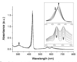
**Figure 2.** Changes in the UV–vis absorption spectra of a toluene solution of  $Sn(TTP)(DTE)_2$  (5 × 10<sup>-6</sup> M) upon irradiation with 365 nm light. Inset shows enlargements of Soret (top) and Q-bands (bottom) regions. The solution was irradiated for 10 s intervals up to 80 s.
