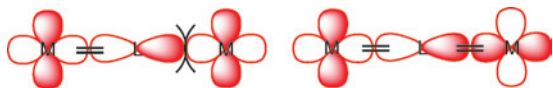
Figure 3. Interaction of a p orbital of a linear bridging ligand with gerade (left-hand side) and ungerade d orbital combinations. Bonding and antibonding interactions are indicated by double straight lines and circle arcs, respectively. The net M–L interaction for the left-hand figure is thus exactly zero.
