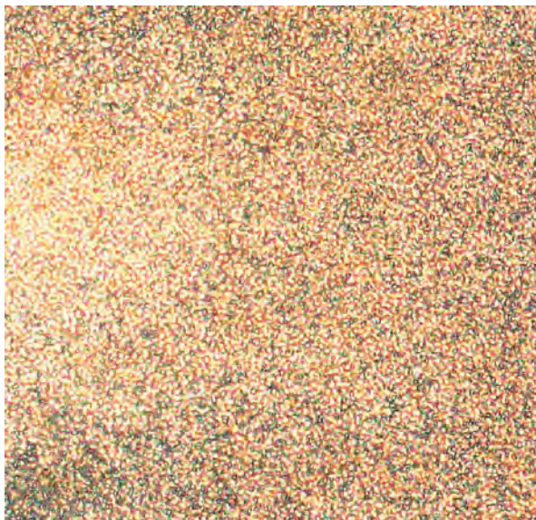
Figure 2. Polarized optical microscopic image of the SmC sanded Schlieren texture (100 \times ) observed for 9c at room temperature.
