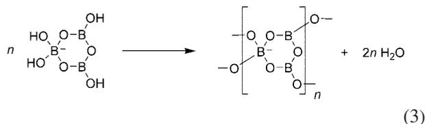
Compound **2** exhibits weight loss of about 16% in the 110–170 °C range, corresponding to the loss of 5 mol equiv of water. This includes both interstitial water and water resulting from condensation of hydroxyl groups. Gradual weight loss continues to about 400 °C, at which point the viscous char begins to darken and puff, apparently as a result of ethanolamine pyrolysis.
