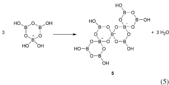
the traborate monoanion, hexaborate dianion (**4**), and nonaborate trianion (**5**), a monocation,  $M^+$ , and no interstitial water have compositions  $M_2O \cdot 3B_2O_3 \cdot 4H_2O$ ,  $M_2O \cdot 3B_2O_3 \cdot 3H_2O$ , and  $M_2O \cdot 3B_2O_3 \cdot 2H_2O$ , respectively.
