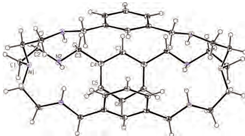
Figure 1. ORTEP diagram of L^2 \cdot MeOH with atom numbering scheme (40% probability factor for the thermal ellipsoid and lattice methanol molecule is omitted for clarity), N_{bridgehead}-N_{bridgehead} distance = 10.913 Å, and the distance between any two secondary nitrogen centers of the tren cavities is 4.033 Å.
