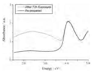
**Figure 12.** Kubelka–Munk absorption spectra of as-prepared AgScO<sub>2</sub> before and after exposure to visible light for 72 h.
