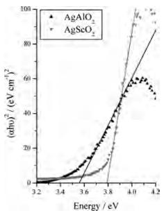
**Figure 6.** Plot of  $(\alpha h v)^2$  versus hv for AgAlO<sub>2</sub> (black) and AgScO<sub>2</sub> (gray). The absorption coefficient  $(\alpha)$  is estimated by the Kubelka–Munk conversion of diffuse reflectance.
