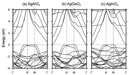
Figure 9. Calculated band structure for (a) AgAlO<sub>2</sub>, (b) AgGaO<sub>2</sub>, and (c) AgInO<sub>2</sub>. Energy zero is at the highest valence band at M.
