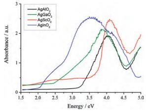
**Figure 5.** Kubelka–Munk absorption spectra of as-prepared silver delafossites.
