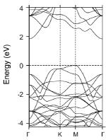
**Figure 10.** Calculated band structure for AgScO<sub>2</sub>. Energy zero is at the highest valence band at M.
