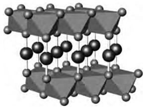
**Figure 1.** Schematic representation of the delafossite structure (ABO<sub>2</sub>). The gray polyhedra and black spheres represent edge-shared B3+O6 distorted octahedra and linearly coordinated A<sup>+</sup> cations, respectively.
