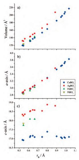
**Figure 8.** Graph illustrating the relationship between the ionic radius of the B-site cation and (a) the unit cell volume, (b) the a-axis length, and (c) the c-axis length for delafossites.
