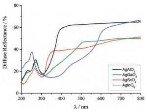
Figure 4. Diffuse-reflectance spectra of as-prepared silver delafossites.
