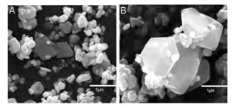
**Figure 2.** SEM images for (a) a mixture of AgScO<sub>2</sub> crystallites ranging in size from a few tenths of one micron up to  $\sim$ 5  $\mu$ m and (b) a close-up view of some micron-sized hexagonal plates of AgGaO<sub>2</sub>.
