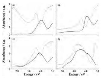
**Figure 7.** Kubelka–Munk absorption spectra of as-prepared silver delafossites (black lines) compared to their corresponding copper delafossites (gray lines) shown for (a) AAlO<sub>2</sub>, (b) AScO<sub>2</sub>, (c) AGaO<sub>2</sub>, and (d) AInO<sub>2</sub>.
