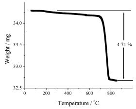
**Figure 3.** Plot of the TGA of AgAlO<sub>2</sub> reduced in a  $N_2$  atmosphere. The final products (verified by XRD) were  $Al_2O_3$  and silver metal.
