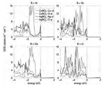
**Figure 11.** Projected densities of A d and O p states for (a)  $AAlO_2$ , (b)  $AScO_2$ , (c)  $AGaO_2$ , and (d)  $AInO_2$ , where A = Cu (gray lines) or Ag (black lines). In these plots, the top of the valence band is taken as zero on the energy axis.
