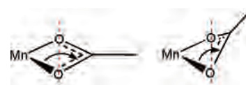
Figure 6. Folding around the O–O vector (red dotted line) decreases the Mn–O–C angle.
