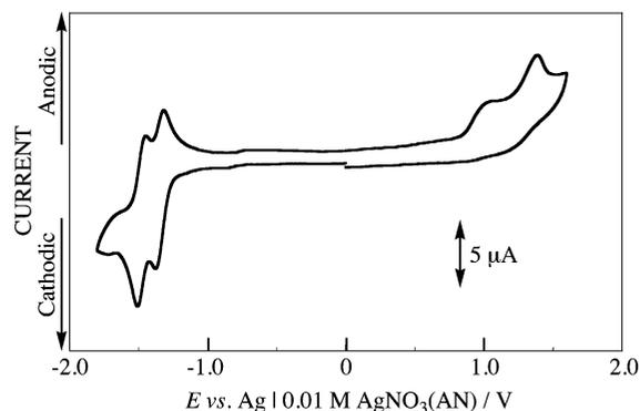
**Figure 1.** Cyclic voltammogram of [{Ru(OCH<sub>3</sub>)(pyca)(bpy)}<sub>2</sub>(μ-N)]PF<sub>6</sub> in  $\text{CH}_3\text{CN}$  at -40 °C.
