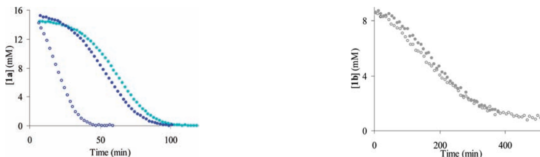
Figure 9. Reaction profiles show that the autoxidation of 1a with no added product (blue filled circles) is slower than with 4 mM added 2a (blue open circles), while 5 mM added 3a (turquoise filled circles) has little effect. Reaction conditions: 11 atm of O_2 and 0.10 mM AIBN in C_6D_6 at 323 K.
