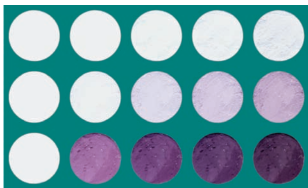
Figure 5. Color of 1 (first row), 2 (second row), and 4 (third row) after 0, 5, 20, 50, and 140 min irradiation (from left to right) at 365 nm. 2 and 3 display very similar optical behaviors.
