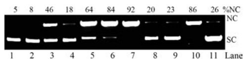
Figure 7. Gel electrophoresis diagram showing cleavage of SC pUC19 DNA ( 0.2 \mu\text{g} , 30 \mu\text{M} ) by complexes 1–5 ( 5 \mu\text{M} ) in the presence of 3-mercaptopropionic acid (MPA, 0.5 \text{ mM} ) in the dark: lane 1, DNA control; lane 2, DNA + 3 ; lane 3, DNA + 1 + MPA; lane 4, DNA + 2 + MPA; lane 5, DNA + 3 + MPA; lane 6, DNA + 4 + MPA; lane 7, DNA + 5 + MPA; lane 8, DNA + distamycin ( 10 \mu\text{M} ) + 3 + MPA; lane 9, DNA + distamycin ( 10 \mu\text{M} ) + 4 + MPA; lane 10, DNA + distamycin ( 10 \mu\text{M} ) + 5 + MPA; lane 11, DNA + methyl green ( 10 \mu\text{M} ) + 5 + MPA.
