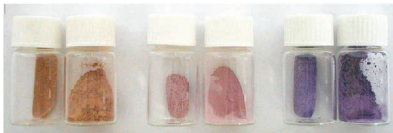
Figure 2. Pumice sheets embedding anhydrous \beta -[Cu(pz) 2 ] n , 2 , (left), hydrated [Cu(pz) 2 ·(H 2 O)] n , 3 , (center), and ammonia complex [Cu(pz) 2 ·(NH 3 )] n , 1 , (right) together with corresponding microcrystalline powdered compounds.
