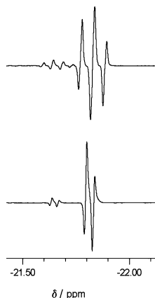
Figure 1. (top) ^1\text{H} NMR spectrum of the hydride region of a sample containing [\text{Ir}(\text{COD})(\text{PPh}_3)_2]^+ in \text{CD}_3\text{OD} with ^{15}\text{N} -pyridine under p\text{-H}_2 , (bottom) ^1\text{H}\{^{31}\text{P}\} NMR spectrum.
