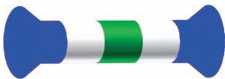
Figure 1. Typical structure of a 1D two-photon chromophore. Two donor parts (blue) are linked to a central core (green) by a conjugated system (white).
