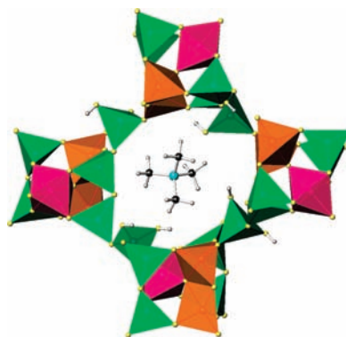
Figure 3. Location of the \text{TMA}^+ ion in the 13-ring channels of PKU-10.
