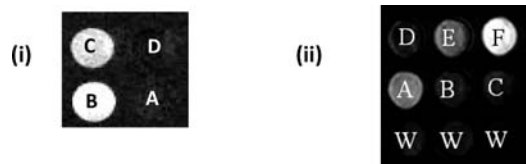
Figure 2. (i) CEST images at 4.7 T of 5.00 mM Yb(S-THP) 3+ in pure water, 25 °C, at different pH values: (A) pure water as a control, (B) pH 4.5, (C) pH 5.5, (D) pH 7.0. (ii) Lower row from left to right: water as control (W). Middle row from left to right: 5.00 mM Yb(S-THP) 3+ , 20.0 mM buffer, and 100 mM NaCl at pH 4.6 (A), 5.5 (B), and 7.0 (C). Upper row from left to right: Addition of 10.0 mM DEP to 5.00 mM Yb(S-THP) 3+ , 20.0 mM buffer, and 100 mM NaCl at pH 4.6 (D), 5.5 (E), and 7.0 (F).
