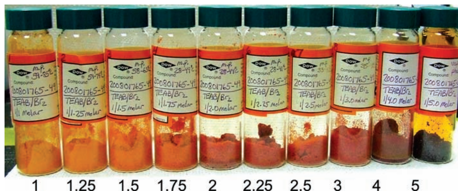
Figure 1. Series of tetraethylammonium polybromide samples prepared via gas-phase reactions. The numbers below each sample refer to the molar ratios of \text{Br}_2 to \text{Et}_4\text{NBr} .
