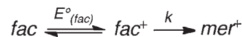
Figure 8. EC mechanism for the oxidation of fac -[(dppe)Mn(CO) 3 Br] which results in the formation of the mer -[(dppe)Mn(CO) 3 Br] + cation.
